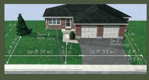
A detailed site plan drawn to scale will help foresee design and construction challenges and provide an accurate reference for estimating. This will become your working or approved plans for the project.
