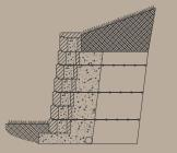
**Chart Example:** A 5 ft. (1.5 m) tall wall in sandy soil with a level surface above can be built with AB Stones of the AB Collection and would typically not require reinforcement, but will require review by a local professional engineer.
