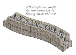
Parapet graphics are to show facing unit and AB Dogbone placements. All parapet installations need to include wall rock in cores.
