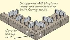
Parapet graphics are to show facing unit and AB Dogbone placements. All parapet installations need to include wall rock in cores.
