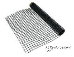
AB Reinforcement Grid is bi-axial (strong in both directions) and can be simply rolled out along the wall. Other geogrids are uni-axial (strong in only one direction) and must be installed running from the front of the block to the back of the excavated area.
