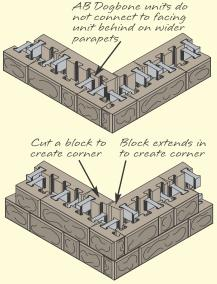
Parapet graphics are to show facing unit and AB Dogbone placements. All parapet installations need to include wall rock in cores.
