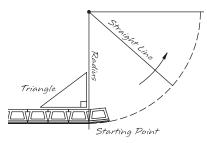
drive a stake into the around. This will be the center of the curve. Attach a string line to the stake the length of the radius and rotate it around to mark the location of the base course. Install the blocks with the front of the blocks lining up with the mark.
